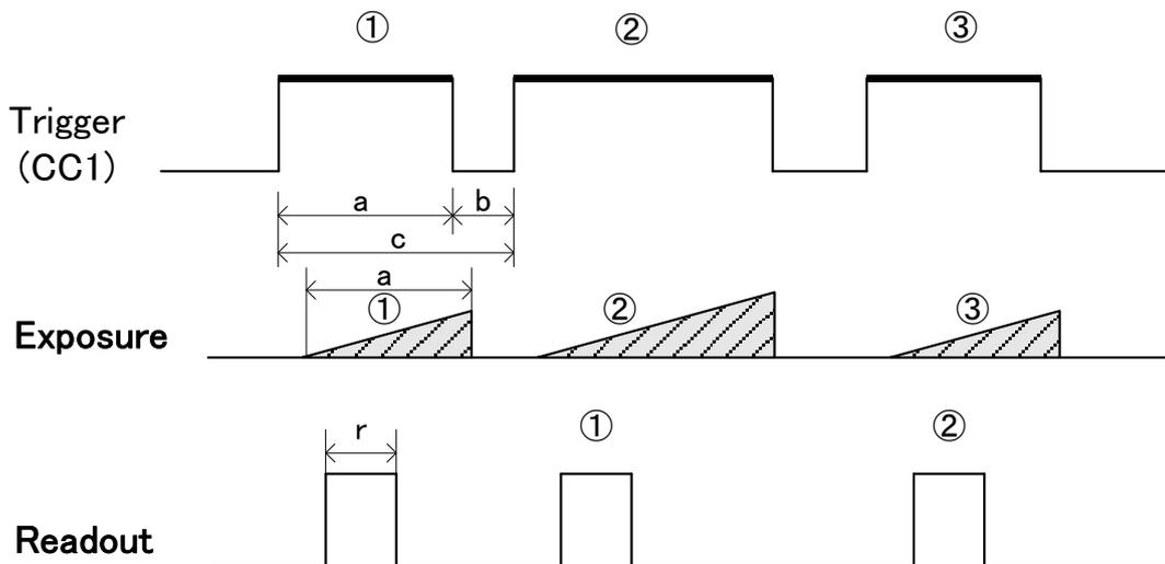
**Figure 4-8-3-1 External Trigger (Trigger Level) Exposure Mode at 4096pixels\_4tap**
