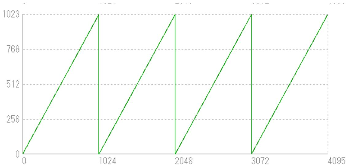
**Figure 4-12-1 Test Pattern of XCM4040DLMT4(4096pixels\_4tap, 4096pixels\_2tap, 4096pixels\_4tap(TypeB))**
