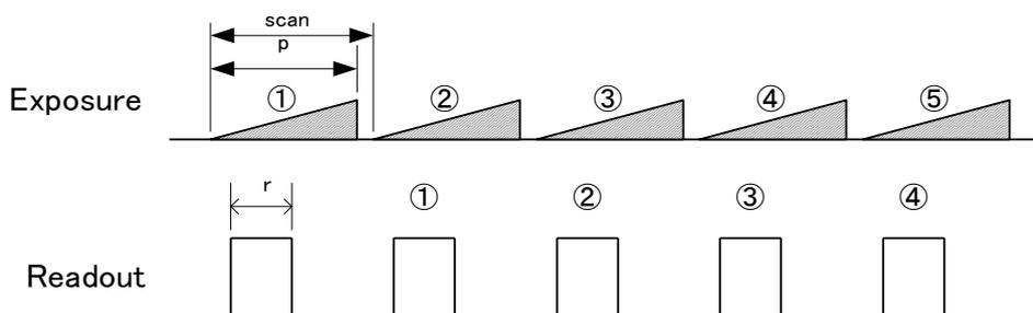
Figure 4-8-1-1 Free Run Exposure Mode at 4096pixels\_4tap
