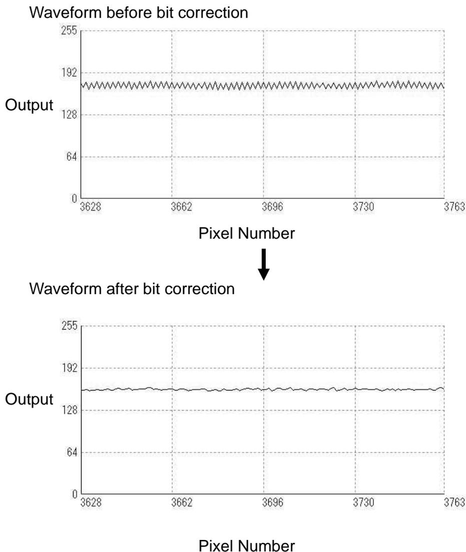
**Figure 4-11-1 Waveform before and after bit correction**
