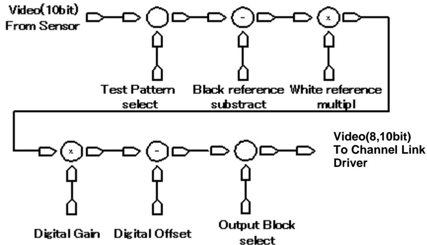
Figure 4-3-1 FPGA Processing Block Diagram
