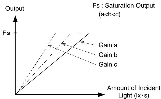
Figure 4-10-1 Gain Adjustment
