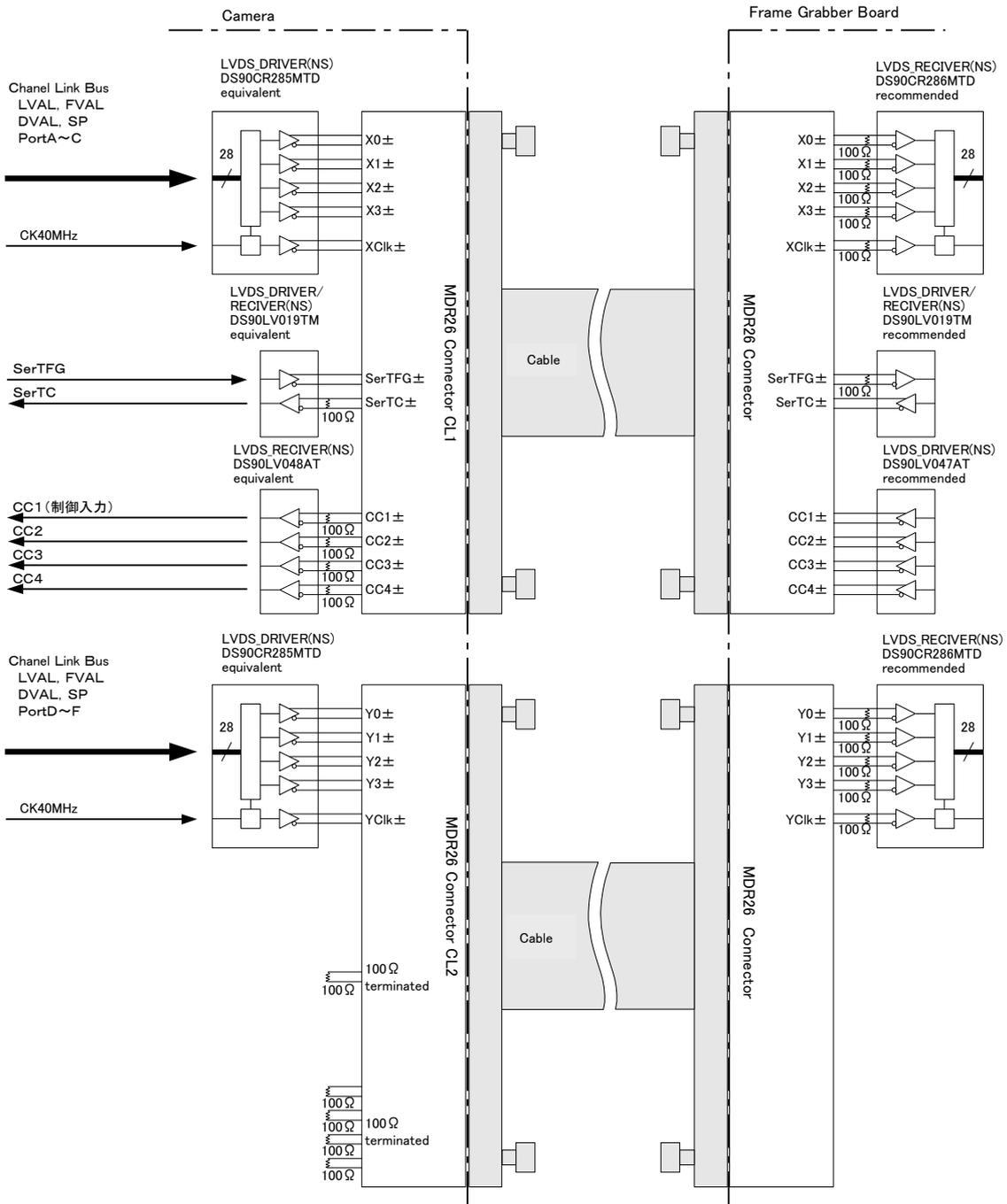
Figure 3-3-1 Camera / Frame Grabber Interface
