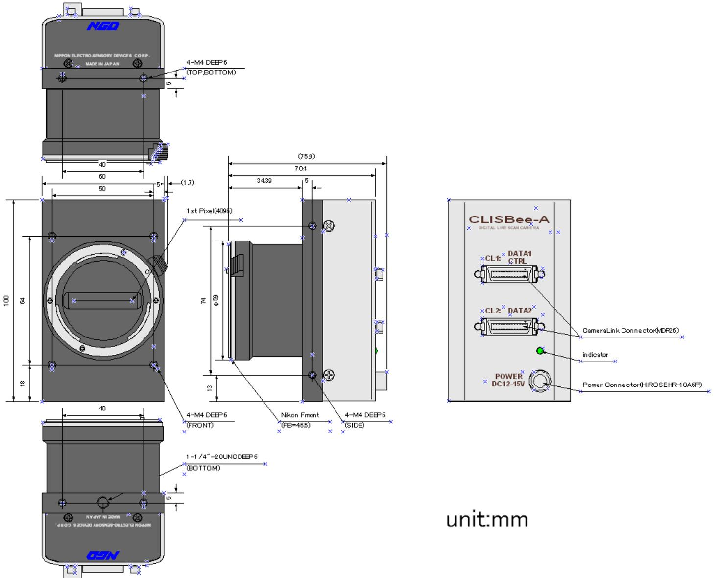
Figure 2-2-1 Dimensions of the Camera
