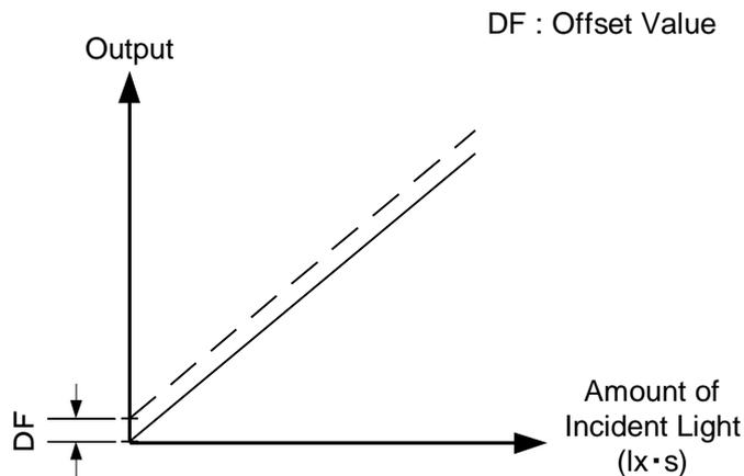
Figure 4-9-2 Offset Adjustment
